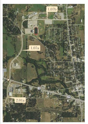
Pojo Road was built in three phases of construction. The portion north of SH 199 was built as a 4-lane roadway facility and the portion south of SH 199 was built as a 3-lane roadway with underground drainage.
